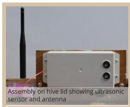
Assembly on hive lid showing ultrasonic sensor and antenna
