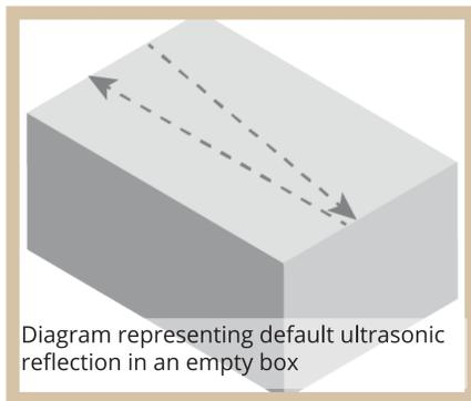
Diagram representing default ultrasonic reflection in an empty box
